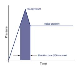
**System pressure** is the differential of pressure between the outlet and inlet ports. It is a dominant operating variable affecting hydraulic unit life. High system pressure, resulting from high load, reduces expected life. System pressure must remain at, or below, rated pressure during normal operation to achieve expected life.
